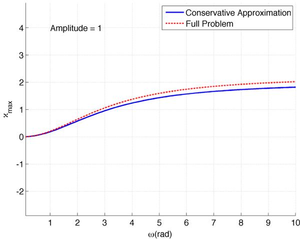
Fig. 8. Comparison of the conservative bound to the full solution for the straight line case. The scanning amplitude was fixed to one unit and the maximum curvature determined as a function of the resolution parameter  $\omega$ . The level of conservatism introduced is small.
