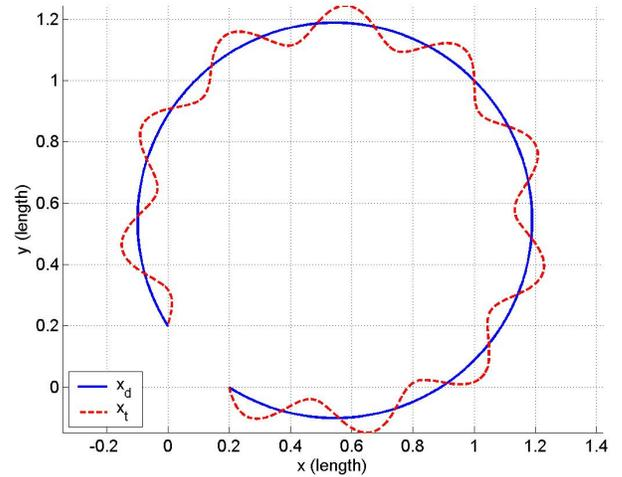
Fig. 2. Example of smooth AFM tip trajectory.  $x_{tip}$  in the dashed line and  $x_d$  in solid line. The amplitude was chosen as  $A = 0.2$ , and the frequency was chosen  $\omega = 10$ . Curvature  $\kappa_d$  was set a constant, making the  $x_d$  a circular path.
