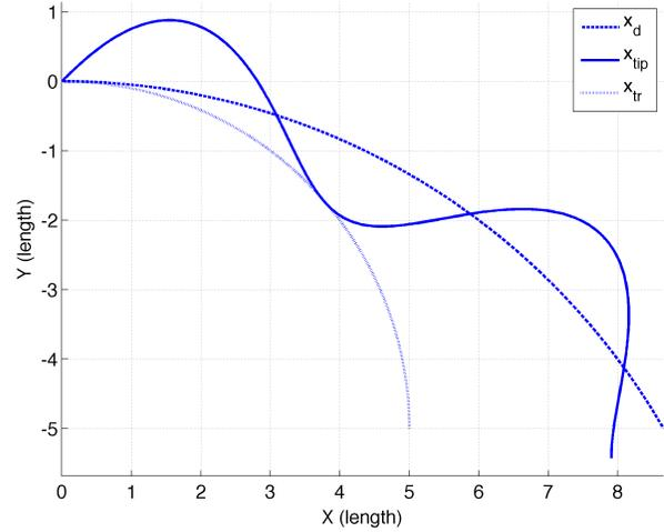
Fig. 4. Full problem setup for the limiting case of tracking a string-like sample. The true sample trajectory, shown dashed, is just about to leave the AFM tip trajectory, shown solid. At this point, the two trajectories must satisfy the “point match” and “tangent match” conditions in (3).
