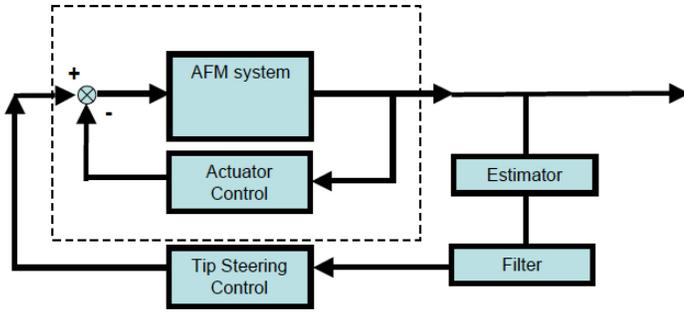
Fig. 1. Feedback control loop of non-raster scanning. The dashed box is the AFM imaging system generating measurement information, which is passed into the feedback loop through an estimator, a filter and a controller to keep the AFM tip around the neighborhood of the string like sample.
