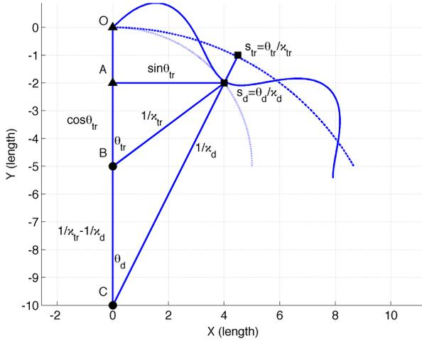
Fig. 5. Geometric relationship between the two arclength parameters  $s_d$  and  $s_{tr}$  using  $\theta_d$  and  $\theta_{tr}$ . In  $\triangle s_d A C$ ,  $\tan \theta_d$  can be found dividing the length  $s_d A = \sin \theta_{tr}$  and  $A C = \cos \theta_{tr} + 1/\kappa_d - 1/\kappa_{tr}$ .
