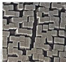
GECKO TAPE Scientists have used diverse materials to make "gecko tapes" that mimic the lizard's remarkable feet. Polyimide gecko tape from Andre Geim's lab at the University of Manchester, in England, is made from a mold created by a lithographic process (above right, each projection is 1 µm long). All Dittmerwalds at Ohio's University of Akron prepared a gecko tape made of columns of carbon nanotubes that has four times the sticking power of gecko feet (left, each column is 100 µm wide).
