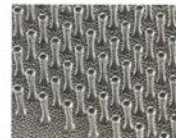
GECKO TAPE Scientists have used diverse materials to make "gecko tapes" that mimic the lizard's remarkable feet. Polyimide gecko tape from Andre Geim's lab at the University of Manchester, in England, is made from a mold created by a lithographic process (above right, each projection is 1 µm long). All Dittmerwalds at Ohio's University of Akron prepared a gecko tape made of columns of carbon nanotubes that has four times the sticking power of gecko feet (left, each column is 100 µm wide).
