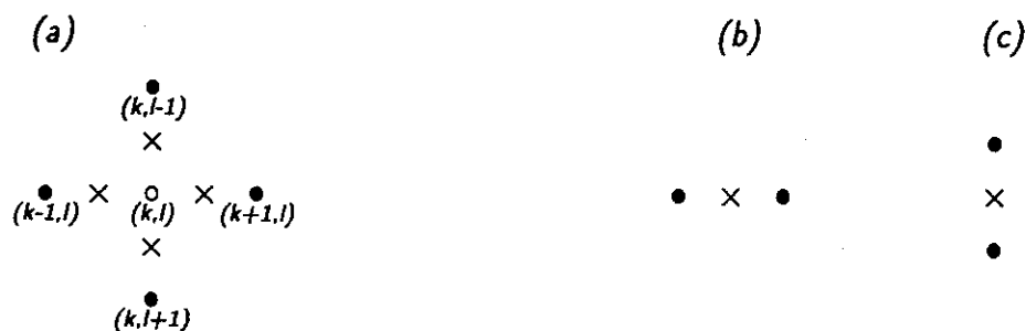
Fig. 6.1 First-order neighbourhood system \mathcal{N}_{(d,l)}^1 for vector field \mathbf{d}_t defined over \Lambda_d with discontinuities (line elements) l_t defined over \Psi_l(a) , and associated horizontal (b) and vertical (c) cliques (o – center vector site, • – vector site, × – line site).
