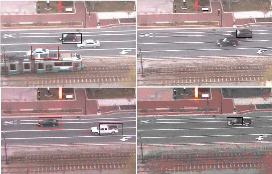
Figure 7: Successful Detection: Red Box for Sedan, Black Box for SUV.
