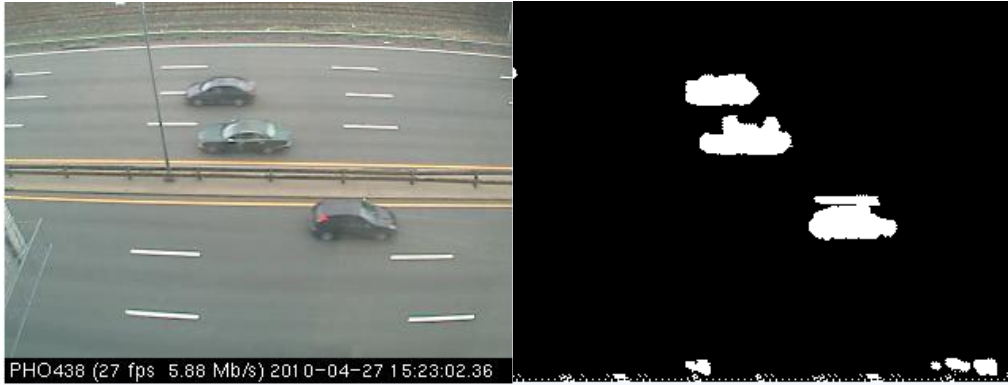
Fig. 16 Applying foreground model to the algorithm
