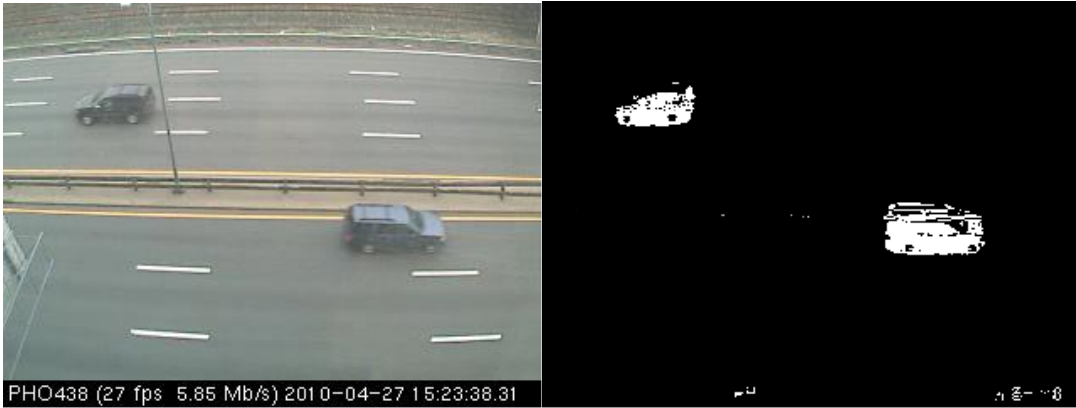
Fig. 8: the result of KDE with LUT and early-break
