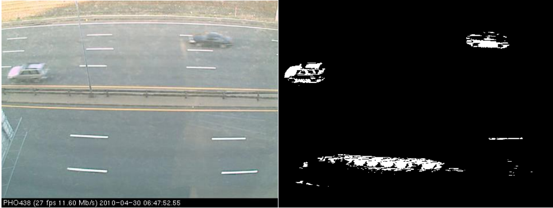
Fig. 5: the result of Single Gaussian Model
