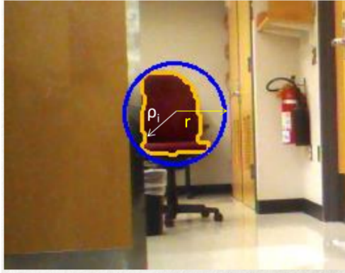
Figure 9: A visual representation of the new error metric. Vector \bar{r} is the radius of the minimum enclosing circle, and vector \bar{\rho}_i is the vector from the center of the minimum enclosing circle to each point.
