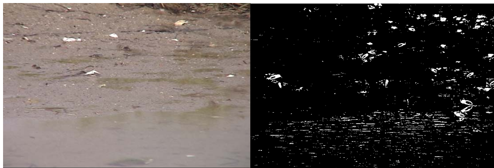
Fig. 1. Frame from original video sequence and result of background subtraction
