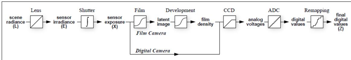
Fig. 3.1 Image Acquisition Pipeline
