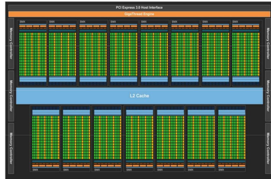
Kepler GK110 Full chip block diagram
