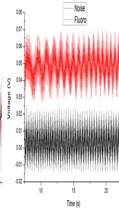
Photovoltage generated by a) commercial UV enhanced Si-PD and b) ZnO nanoparticles-AlGaN substrate detector (back lighting) when the tryptophan enzyme in E-coli(ATCC # 25922) excited by a 280nm LED.
