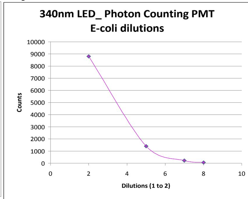
E-coli diluted samples measured in a quartz cuvette with path length of 3 mm by 280 and 340 nm UV LEDs and PMT photon counting module. A 340 nm band pass and 400 nm long pass emission filter was placed in front of the PMT for the 280 nm and 340 nm excitation respectively.
