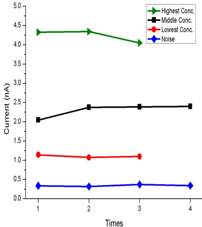
Detection of tryptophan enzyme in E-coli (ATCC # 25922) in different concentration by ZnO nanoparticles-AlGaN substrate detector (back lighting) when the cells is excited by a 280nm LED.
