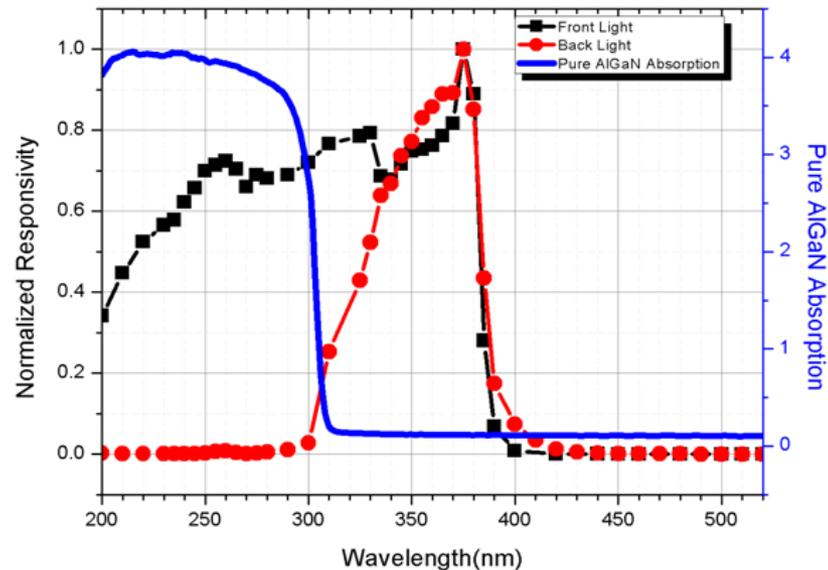
Spectral response of ZnO nanoparticles-AlGaN substrate detector a) Front lighting compared with commercial UV enhanced Si based photodiode and b) Front and back lighting compared with absorption spectrum of AlGaN substrate
