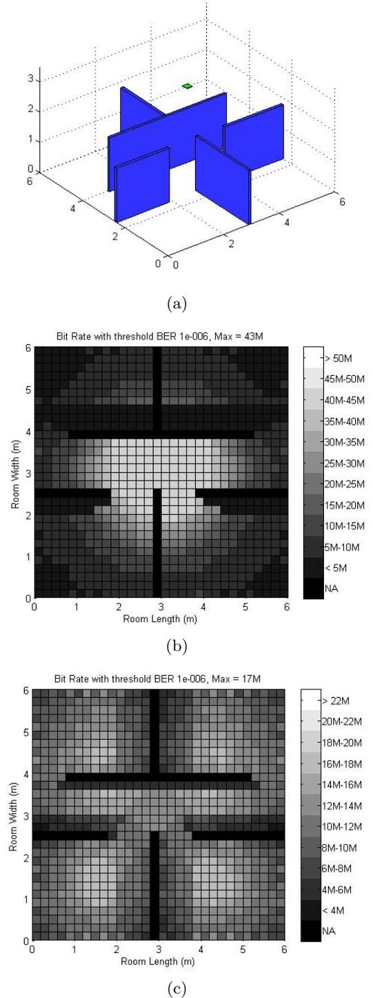
Figure 4: Simulated 4PPM results in a 6m X 6m X 3.5m office for a receiver at a height of 1m with (b) a single 5W transmitter at the center of the ceiling, and (c) four 1.25W transmitters spaced evenly on the ceiling.
