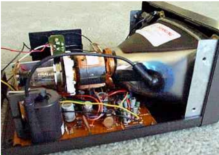
(Note the large black electrode hooked to the tube near the screen -- it is connected internally to the conductive coating.)
