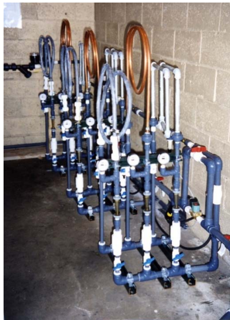
Figure 5.2 Mini-pipe loops of three metals for chemical treatment comparison in 1999
