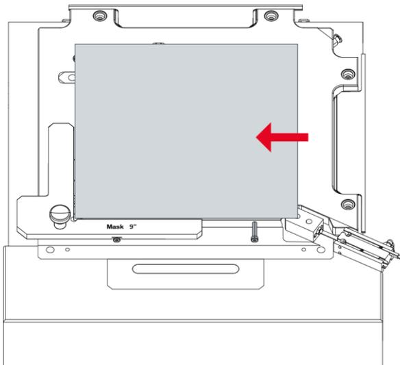
*Fig. 63: Align the substrate*
