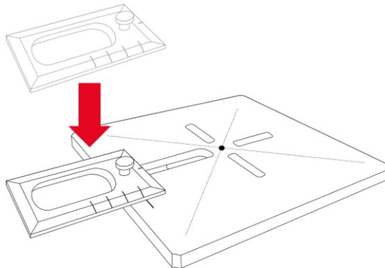
Fig. 57: Place the adjustment aid for medium-sized substrates
