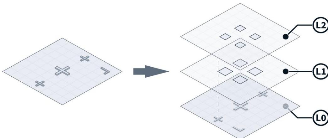
Fig. 12: Backside alignment marks on the lower surface
