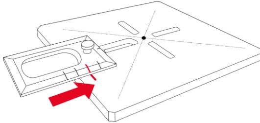
*Fig. 58: Align the adjustment aid*
