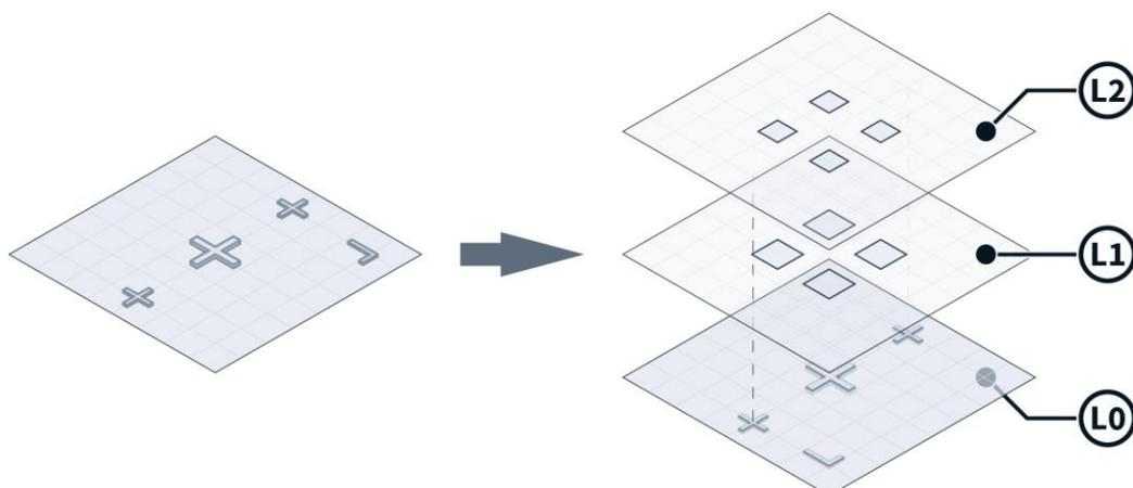
Fig. 74: Backside alignment marks on the lower surface
