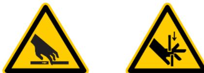
**⚠ Moving mechanisms can be dangerous.** Keep clothing, hands, and body out of the operating area. Do not stand or sit on any part of the machine.
