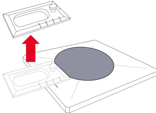
*Fig. 61: Remove the adjustment aid.*
