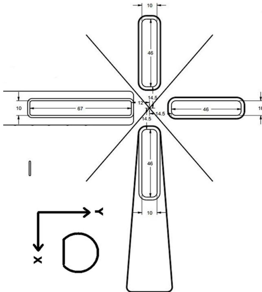
Fig. 13: Chuck – Backside alignment zones (standard chuck layout)
