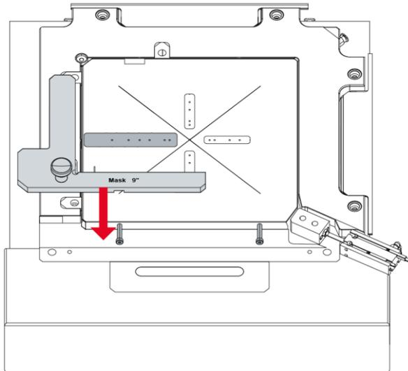
*Fig. 62: Place the adjustment aid for large substrates*
