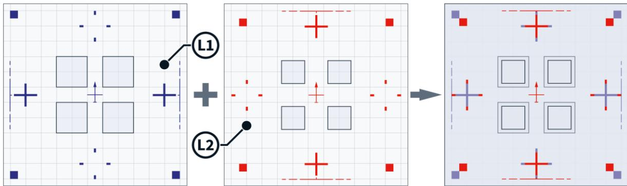
Fig. 73: Example of alignment mark design and placement
