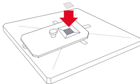
*Fig. 54: Place the substrate in the adjustment aid*
