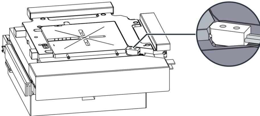
Fig. 68: Pneumatic clamp
