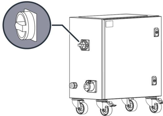
Fig. 51: Main switch at the step-up transformer
