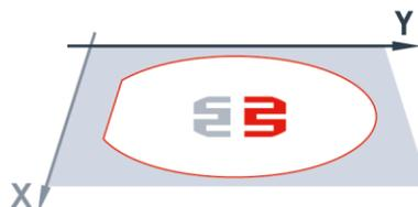
Fig. 10: Stage coordinate system
