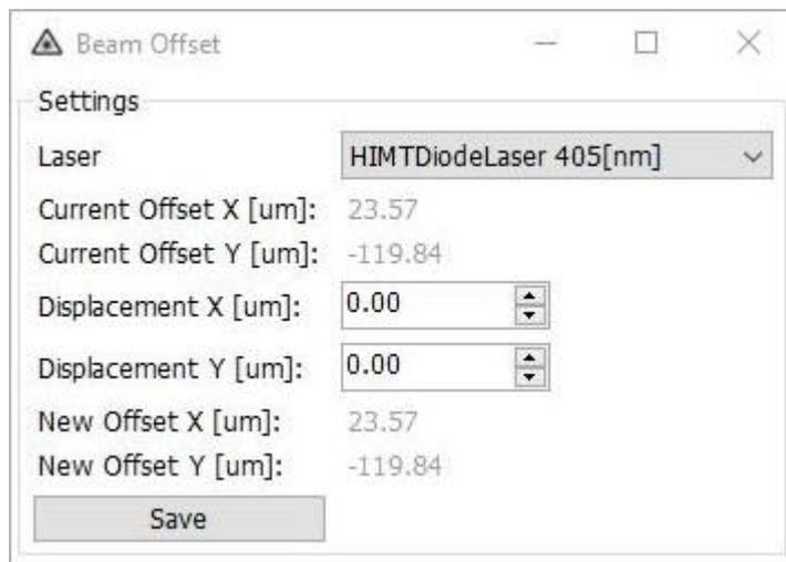
Fig. 96: Beam Offset dialog – Calculated beam offset
