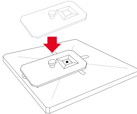
*Fig. 53: Place the adjustment aid for small substrates*
