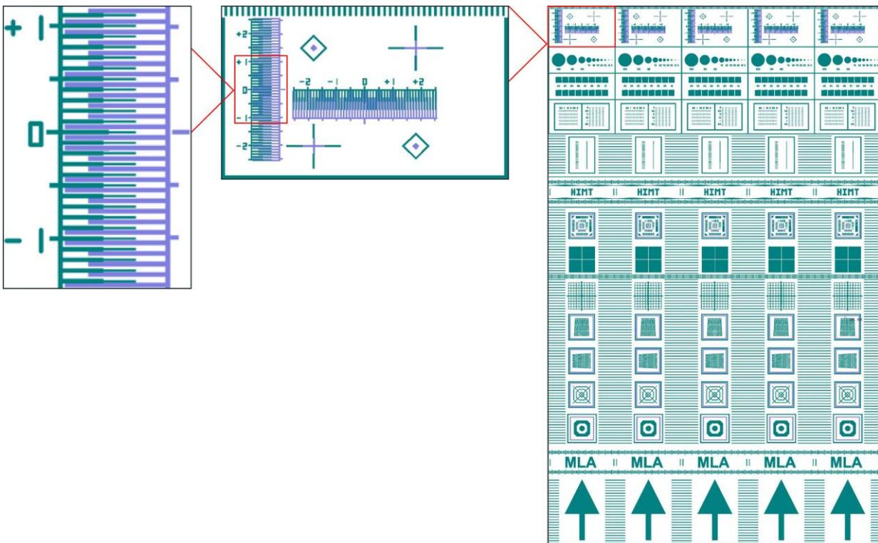
Fig. 95: Vernier scale in FAT test pattern
