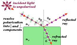
The reflected light mostly contains the perpendicular component of the incident light. At a certain angle of incidence (Brewster's angle), the reflected light is all linearly polarized perpendicular to the plane of incidence. The value of Brewster's angle depends on the indices of refraction of the first and the second medium.
