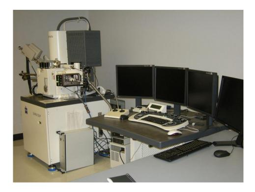
Zeiss Supra 55VP Field Emission Scanning Electron Microscope
