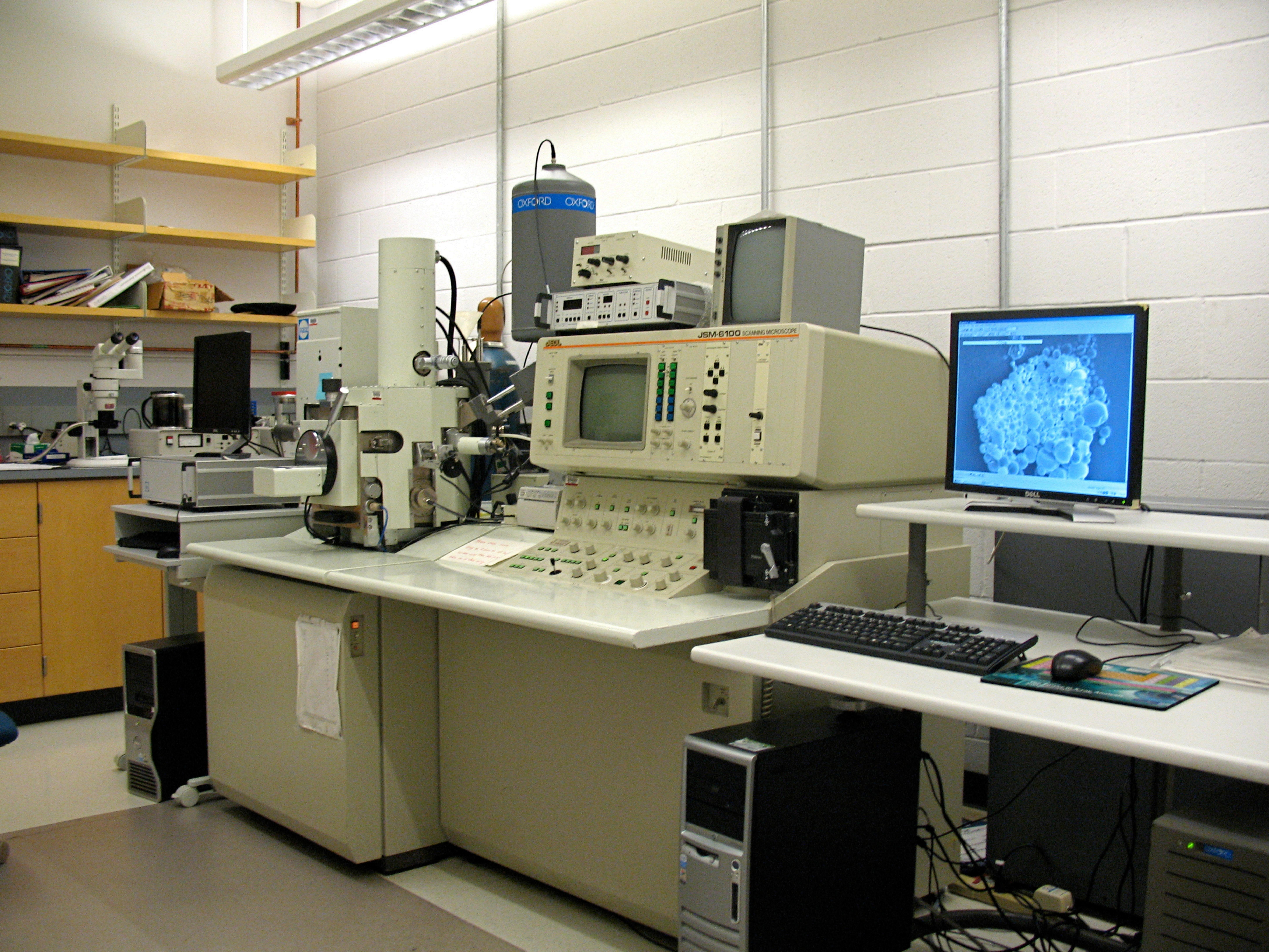
JSM-6100 SCANNING MICROSCOPE
