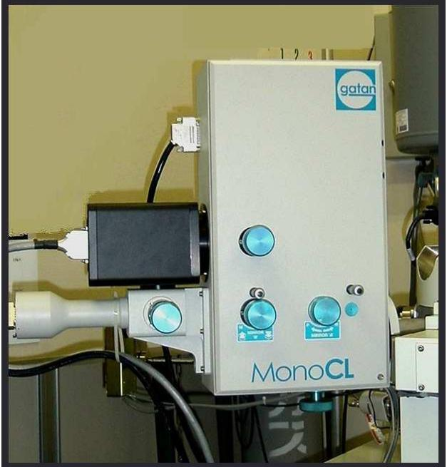
With Gatan's monoCL3 spectroscopy system, high-resolution, cathodoluminescence spectra (range 180nm-800nm) can be collected.
