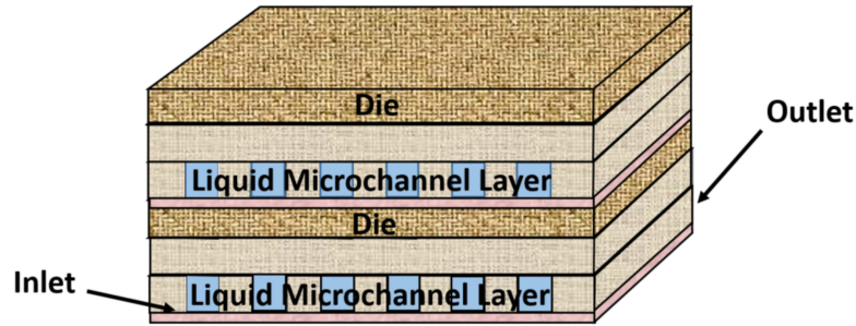
Figure 2-4: Liquid cooling via microchannels 3D IC architecture (Sridhar et al., 2014).
