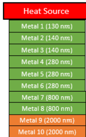
Figure 3-24: The layer stack of the interconnect model.
