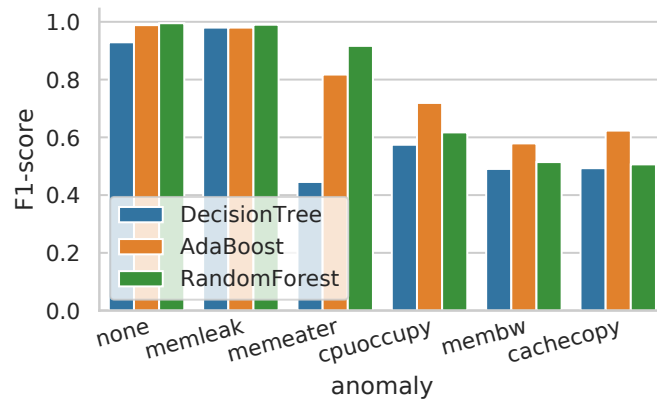
Figure 5-9: Results for classification of the anomalies. The overall F1-score using Random Forest algorithm is 0.94.
