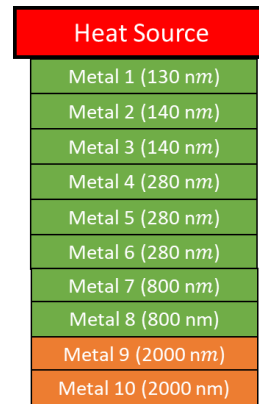
FIGURE 4: THE LAYER STACK OF THE INTERCONNECT MODEL.
