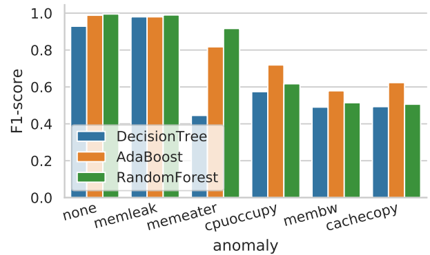
Figure 9: Results for classification of the anomalies. The overall F1-score using Random Forest algorithm is 0.94.
