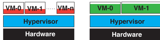
a) Server w/ Enterprise Workload b) Server w/ HPC-type Workload Fig. 1. Virtualized server illustration for a) enterprise workloads and b) HPC-type workloads.
