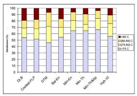
Fig. 1. Distribution of Thermal Hot Spots, with DPM
