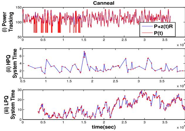
Fig. 5. Power-performance profiles of Canneal with  $\bar{P} = 113W$  and  $R = 30W$ . (i)  $\bar{P} + z(t)R$  and  $P(t)$  trajectories (in Watts). The tracking error statistics:  $\bar{\epsilon} = 0.09$ ,  $\sigma_{\epsilon} = 0.40$ . (ii) HPQ system time degradation trajectory with overall statistics:  $\bar{d}_{can}^H = 3.03$ ,  $\sigma_{d_{can}^H} = 1.28$ . (iii) LPQ system time degradation trajectory with overall statistics:  $\bar{d}_{can}^L = 13.05$ ,  $\sigma_{d_{can}^L} = 7.28$ .
