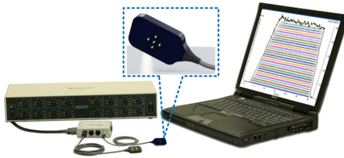
Figure 1. The sEMG sensor, the signal acquisition and amplification unit and a PC loaded with the decomposition algorithm are shown. The pins on the sEMG sensor are 1.25 mm long and approximately 0.57 mm in diameter; four of which are located at the corner of a 5 mm 2 , and one in the center of the square.
