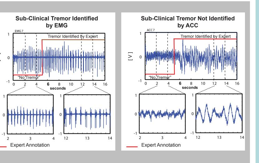
Sample data from a patient asked to sit quietly. The left figure indicates the "Off" period when the patient experienced Tremor, and the right figure indicates the "On w/ Dyskinesia" period. Data were recorded from the Anterior Deltoid and Biceps brachii muscles. EMG signals are in black; ACC signals are in blue.
