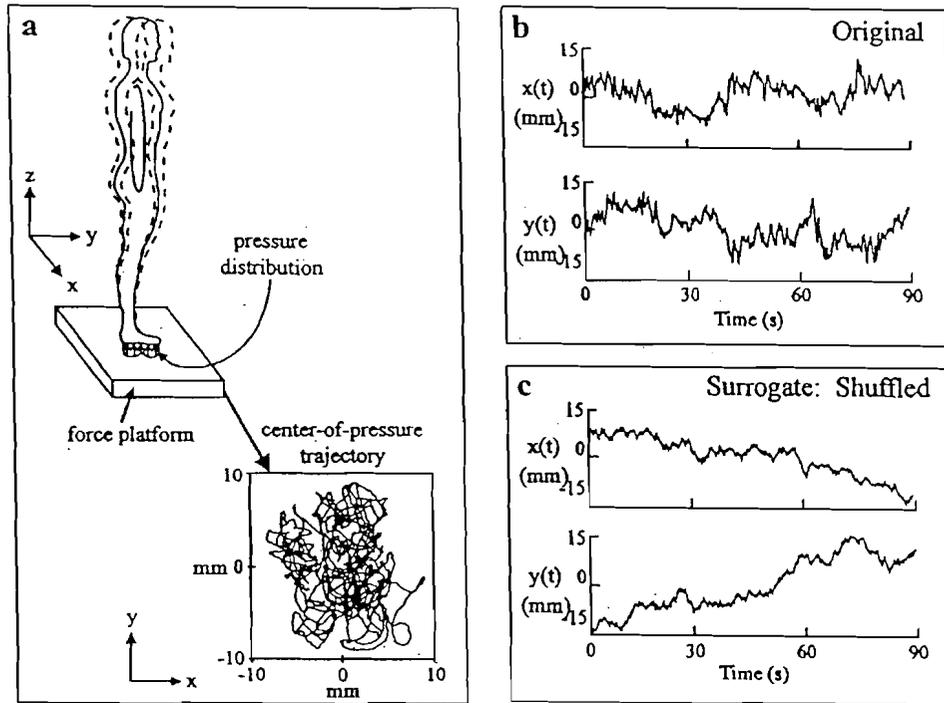
FIG. 1. (a) A schematic diagram of the experimental setup for examining quiet-standing postural stability. Shown also is a typical 90 s stabilogram for a healthy young individual. (b) The  $x$ -coordinate and  $y$ -coordinate time series corresponding to the stabilogram in (a). (c) Shuffled surrogate random-walk data sets that were generated from the original COP time series in (b).
