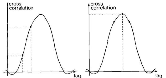
FIG. 2. Illustration of conduction velocity estimation method. Cross-correlation function of 2 myoelectric derivations and initial lags of cross-correlation estimation (left). Difference of cross-correlation values at 2 nonadjacent lags is used in a feedback loop to control delay lines of conduction velocity estimation. After convergence, lags are properly positioned (right), and time to middle lag is used as time to maximum of cross-correlation function.
