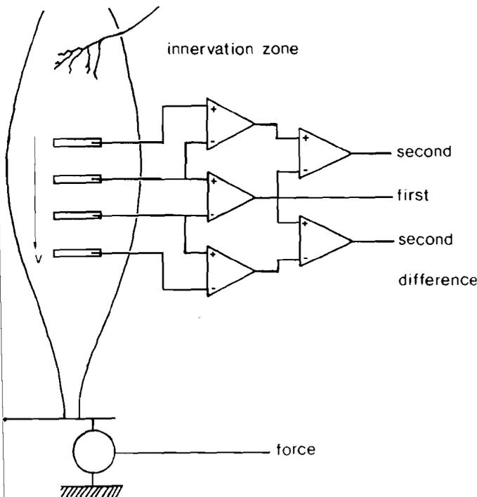
FIG. 1. Schematic of detection setup. Electrode unit with 4 bars, separated by 1 cm, is placed on 1 side of innervation zone. 3 myoelectric signals, 1 first differential and 2 second differentials, are recorded for further off-line processing. Force transducer output is also recorded.
