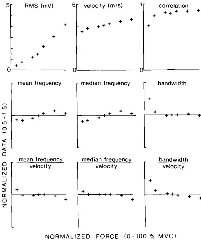
FIG. 5. Means across subjects of parameters from force study. Spectral parameters are from first differential myoelectric signal. Parameters shown are as follows: First row: root-mean-square (rms) value, conduction velocity, and maximal correlation; Second row: Normalized mean frequency, normalized median frequency, and normalized bandwidth; Bottom row: parameters of second row divided by normalized velocity.
