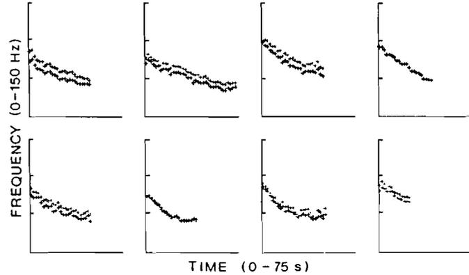
FIG. 10. Means across subjects of mean (*top*) and median (*bottom*) frequencies vs. time during a sustained high-force-level contraction (nominally 80% MVC). As endurance time varied across subjects, plotted data represent means across a varying number of subjects. Data were obtained from first differential myoelectric signal.
