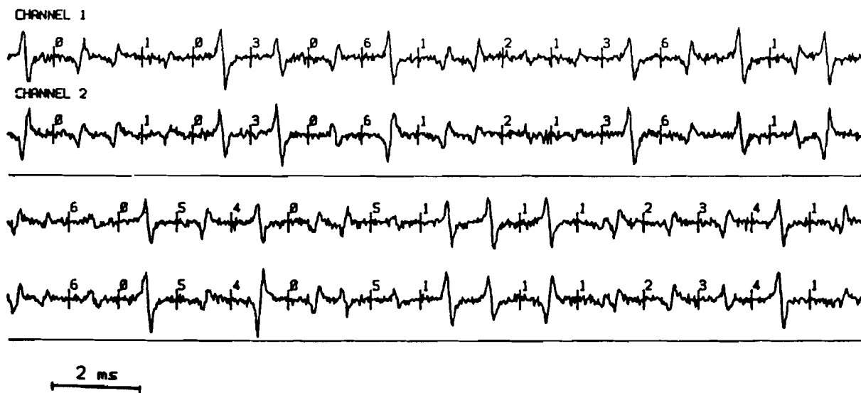
Fig. 6. An example of mathematically synthesized and time compressed EMG signal used to test the accuracy of the decomposition system. As in the previous figure, the vertical lines are skipped interval markers and the numbers represent the milliseconds of time removed.
