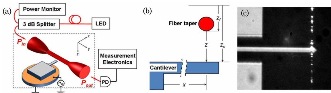
Fig. 1. (Color online) (a) Schematic of the experimental setup. (b) Cross-sectional view showing the coordinate system. (c) Microscope image of the fiber taper and microcantilever. Visible light is passed through the fiber taper in this image.
