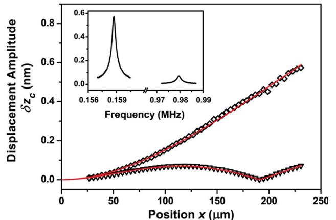
Fig. 3. (Color online) Displacement amplitudes in the first two out-of-plane modes of the microcantilever measured by positioning the fiber taper along the length of the microcantilever. Solid curves are fits obtained from theoretical calculations. The inset shows the resonance line shapes measured close to the free end of the microcantilever. For all the measurements, the dc component of  $P_{\text{out}}$  is  $\sim 32 \mu\text{W}$ .
