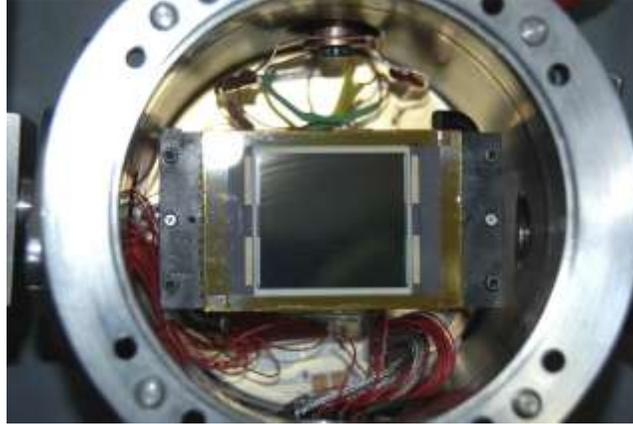
The new science array for PRISM installed in the dewar.
