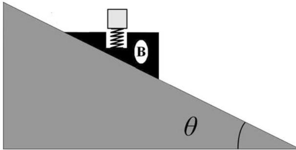
**Fig. 3** Box *B* slides frictionless on the incline and supports a weight sensor by means of which the body's weight in motion is measured
