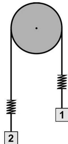
**Fig. 13** Schema of Atwood machine with weighing devices and further extra masses
