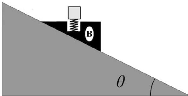
**Fig. 3** Box B slides frictionless on the incline and supports a weight sensor by means of which the body's weight in motion is measured
