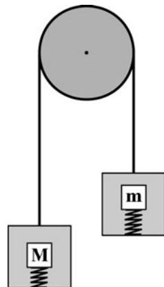
You can show that the weights of the two blocks are 13 N ( $=mg$ ) and 27 N ( $=Mg$ ). So the tension ( $=17$  N) does indeed lie between these two values (Halliday et al. 1993, p. 116).
