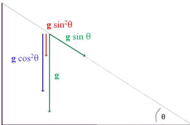
**Fig. 4** The vertical component of the acceleration of the box is represented in red and inside the *box* in blue. (Color figure online)
