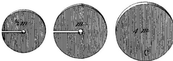
**Fig. 17** Three pieces used to vary the weight of the boxes (Atwood 1784, fig. 81, 80, 79). The symbol “m” on the pieces does not represent mass but rather weight,  $m = \frac{1}{4}$  oz
