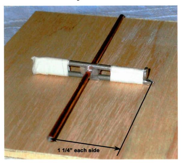
The electromagnet is made by wrapping the magnet wire onto the nails.
