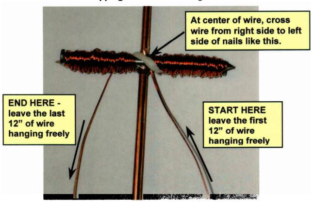
The two ends of the wire coil that you left sticking out are called the electromagnet leads, because they lead electricity into and out of the coil. Magnet wire is painted with enamel paint to insulate the wire, so you must sand the paint off the wire in order to make an electrical connection to the bare copper.
