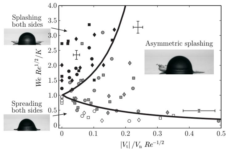
**Figure 5.** Experimental results from figure 4 recast to show global drop behavior. The model predicts three behaviors based on the magnitude of the tangential velocity: the lamella will spread in all directions (white symbols), splash in all directions (black symbols) or asymmetrically splash (gray symbols). Here  $K = 5700$ .
