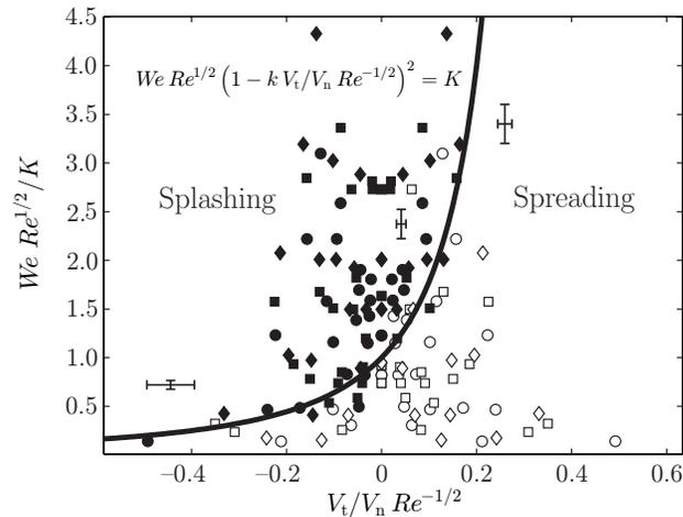
**Figure 4.** Experimental results for ethanol drops with different radii,  $R = 0.88$  mm (○, ●), 1.3 mm (□, ■) and 1.7 mm (◇, ◆), approximately collapse on to a master curve when rescaled according to our theory. The model prediction (solid line) agrees well with the experimental data when  $k = 2.5$  and  $K = 5700$  in equation (5). Representative error bars are placed at three locations.
