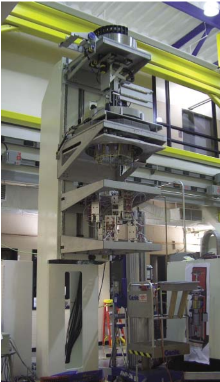
Continuous Crystal Growth System for the Production of Solar Cells.
