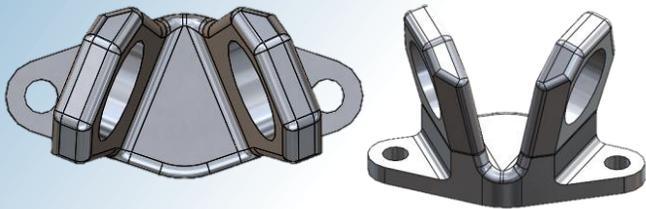
*The 8 load transfer units (4 on bulkhead, 4 on engine mount) will have 3/16" spherical joints press fit in to avoid static indeterminacy*
