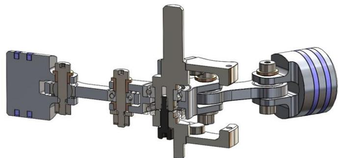
*The center linkage required extensive tribology research, and features spherical joints, misalignment bearings, adjustable counterweights, interference fits, and more*
