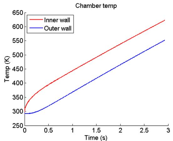
*2.9 sec to reach 350°C at thermal failure point*
