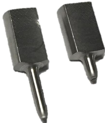
Non-heat treated steel after tensile testing
