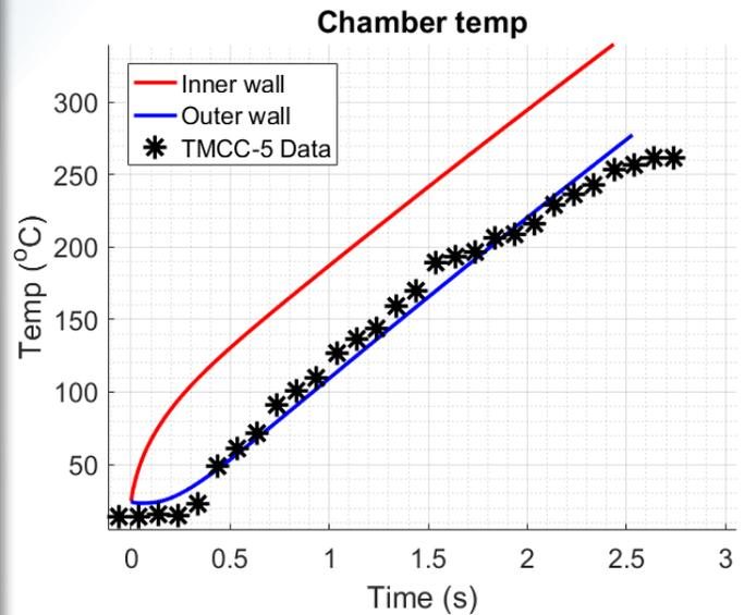
*Thermocouple data closely match temperatures predicted by the thermal model*
