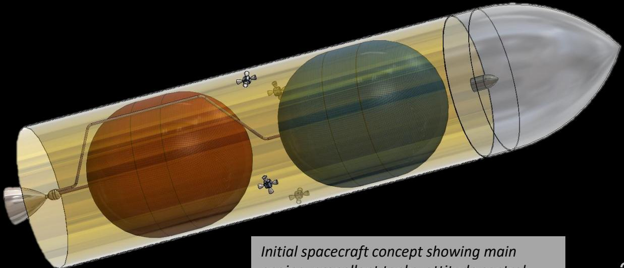
*Initial spacecraft concept showing main engine, propellant tanks, attitude control thruster modules, and tungsten penetrator*
