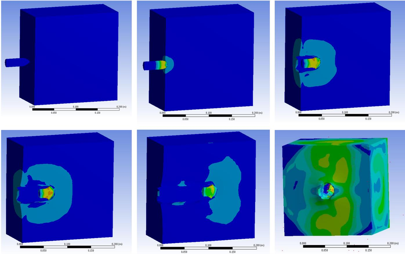
Hypervelocity impact simulations in ANSYS reveal that the stresses involved in a collision directly from orbit are unsurvivable. Retropropulsion would add another 1.43 km/s of required  $\Delta V$  to the spacecraft, but would allow the payload to remain intact.
