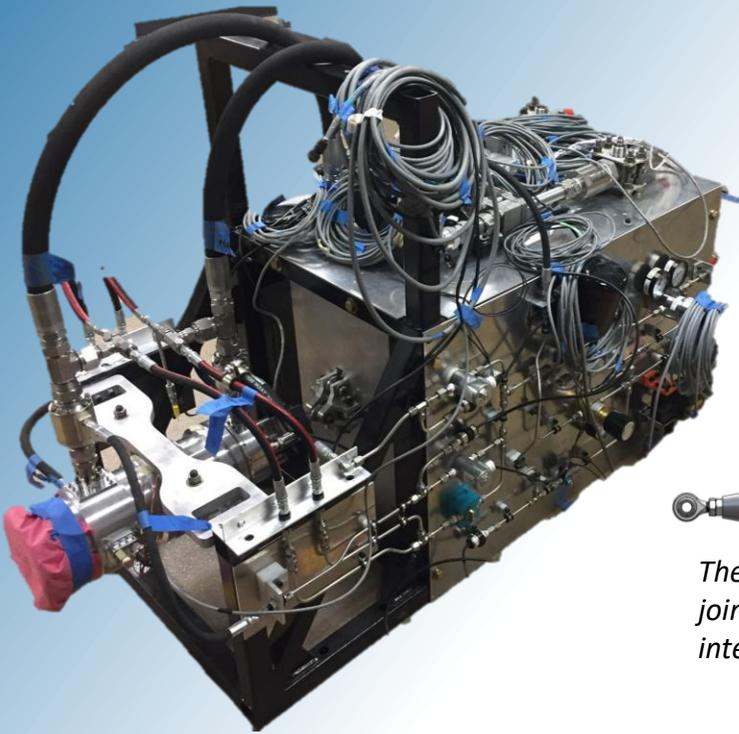
Fully assembled test stand. Engine clevis and thrust plate visible behind LD2 engine
