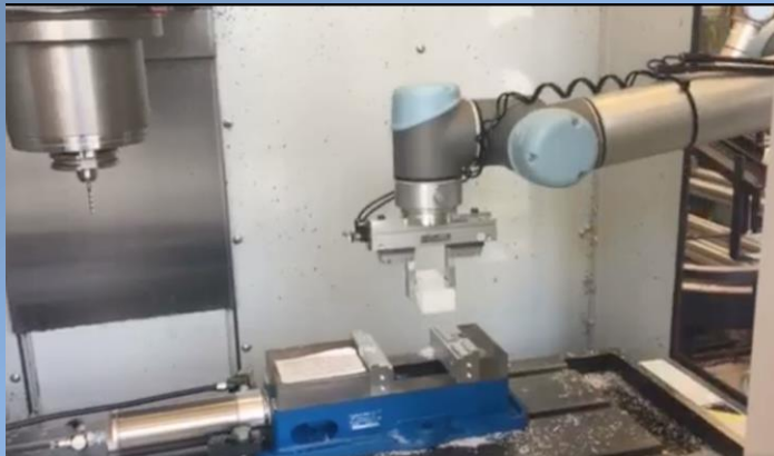
Programmed Robot loading stock into CNC Mill
