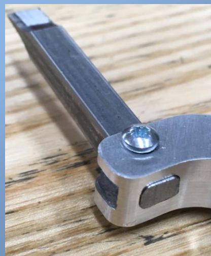
Screwdriver slides into slot to prevent excessive torque on pin
