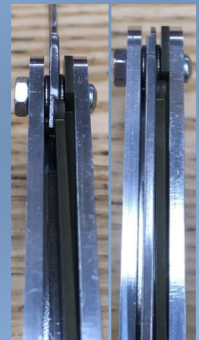
Liner lock snaps into place to keep knife open (L) and holds against blade with friction to keep it closed (R)
