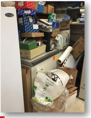
Deficiency: Flammable chemicals not stored in flammable cabinets when not in use
