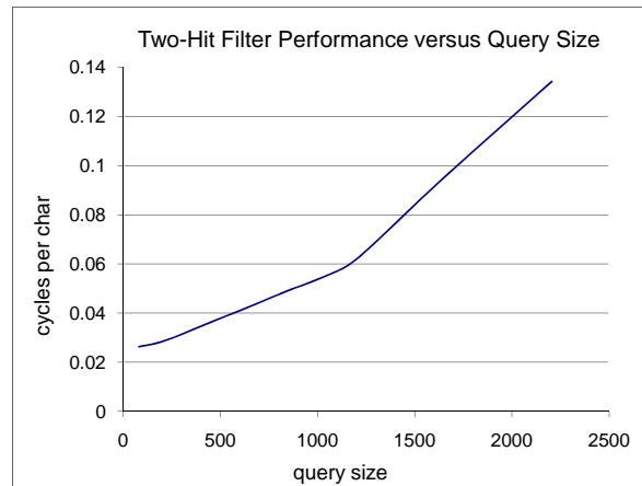
Figure 7: Graph shows performance as a function of query size for the Two-Hit filter in the reference design. Both the number of filters and the throughput per filter vary with query size.
