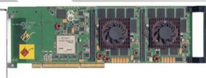
Shown is the WildstarII-Pro board from Annapolis Micro Systems, Inc, with two Xilinx Virtex-II-Pro XC2VP70-5 FPGAs.
