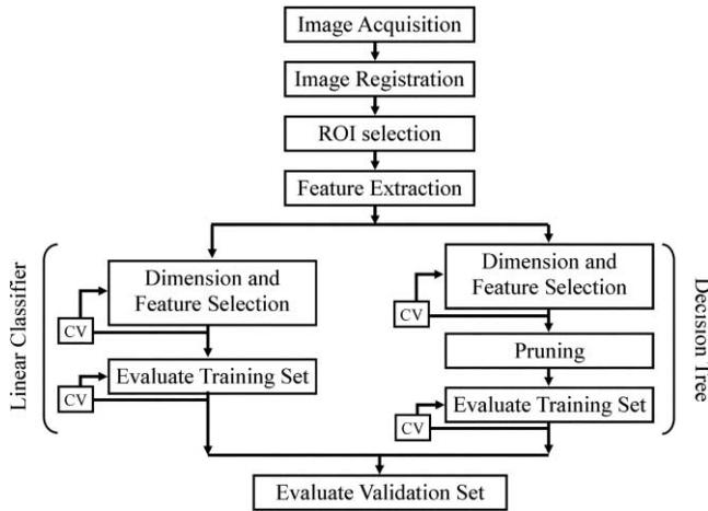
**Fig. 2** Flowchart of computer-aided diagnostics procedure. CV denotes cross-validation.
