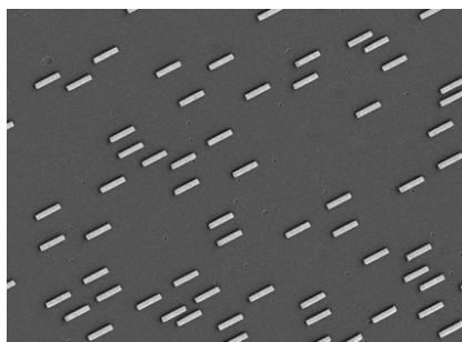
Molecules consist of atoms connected to each other by bonds (top), which vibrate at specific resonant frequencies. BU researchers engineered rod-shaped gold nano-antennae (bottom) to increase the vibration signals coming from biomolecules.
