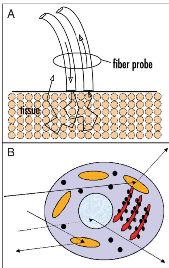
Figure 2. (A) The optical geometry for delivery and collection fibers for a typical “optical biopsy” measurement. The fiber probe is placed in gentle contact with the tissue surface; (B) cartoon depicting the scattering of photons by denser organelles and nucleus in the cell.
