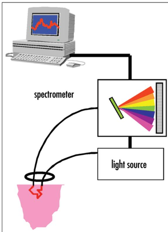
Figure 3. System components for elastic scattering spectroscopy.
