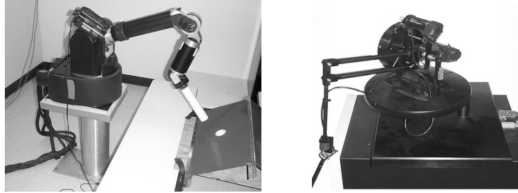
Figure 2. (a) WAM remote robot arm with connector mating apparatus. (b) PHANToM master arm.
