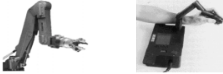
Figure 1. Schilling Robotic Systems Titan II manipulator, one of the leading commercial robots for undersea applications. (a) Remote manipulator arm is hydraulically powered. (b) The passive master arm provides no force feedback.
