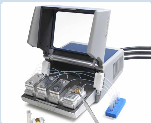
1. Mount quartz crystal sensors in the temperature controlled chamber. Four sensors are fixed in removable flow modules with inlet and outlet. The quartz crystal sensors may be pre-coated with, for example, metals, polymers or SAMs.
