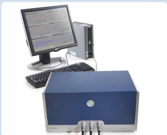
3. Follow results in real time on the computer screen. Frequency changes reflect mass changes taking place on the sensor surface, dissipation changes reflect changes in the adlayer's viscoelastic properties.
