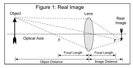
However, the same lens, when placed *close* to an object, produces a magnified *virtual* image which can be seen through the lens with the eye, but cannot be projected onto a screen (see Figure 2). A **negative lens** has at least one concave surface and always produces a virtual image. All of the lenses in this exercise have convex surfaces (the glass surface bulges outward from the lens center).
