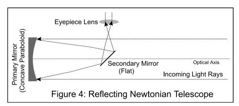
The first telescope design that used mirrors instead of lenses was invented by Isaac 1680. Newton in The objective in this design (see Figure 4) is a concave parabolic mirror, which reflects light onto a flat secondary mirror, moving the focus of the primary outside of the path of the rays entering
