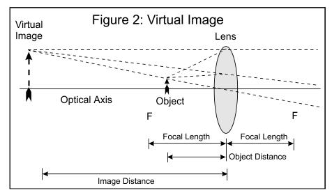
Note: The dashed lines in each figure represent a few of the numerous light rays leaving from a single point on the object. The rays that fall upon the lens are bent to form an image. For simplicity, these diagrams show only three rays from one point at the top of each object.
