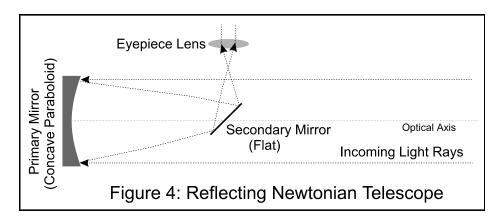
The first telescope design that used mirrors instead of lenses was invented by Isaac Newton 1680. in objective in this design (see Figure 4) is a concave parabolic mirror, which reflects light onto a flat secondary mirror, moving the focus of the primary outside of the path of the light entering rays
