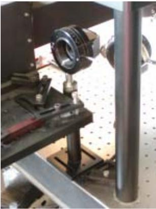
Make sure the 2" lens is not in place, and that the rotator is. The **scanning motor** should be turned off, and the two black lines on it should match, indicating that the image is centered on the slit.
